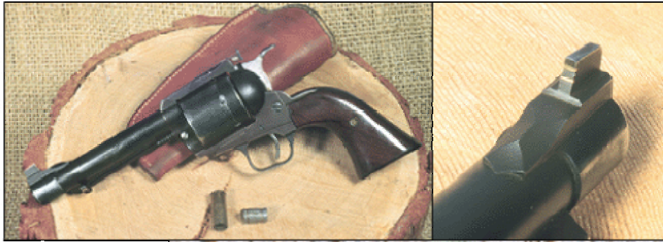
Above, the gun that started it all is a six-shot conversion with oversize cylinder on an El Dorado frame with the case and bullet that finished the buffalo. Above right, the front sight is a completely resculpted front band from a Ruger No. 1 rifle. Right, Ross with Hugo Scia, the buffalo and the "short .458."
